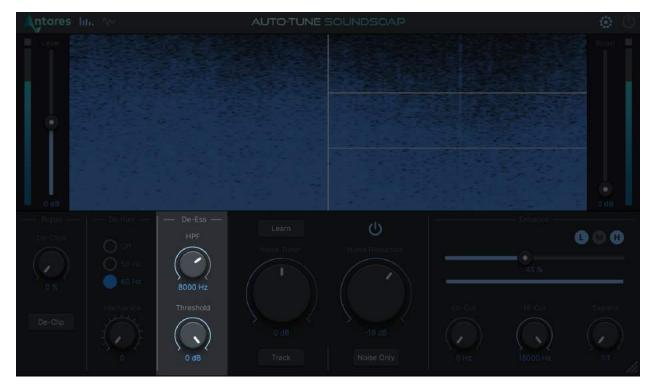
The De-Ess section helps remove audible <u>sibilance</u> from vocal recordings and performances.
