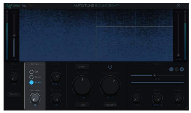
The De-Hum controls help you eliminate unwanted <u>hum</u> in your recordings caused by electrical interference.
