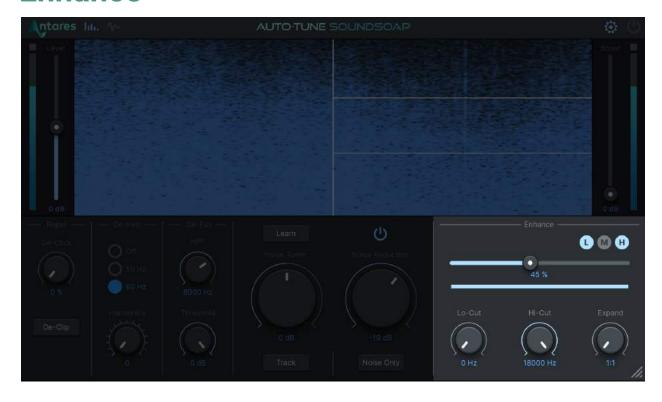
The Enhance Slider adds "sparkle" back into the audio signal by boosting frequencies that may have been lost in degraded media. Use the L, M, and H buttons to toggle which frequencies are boosted by the Enhance slider. You may select up to two frequency ranges to boost.
