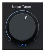
The **Noise Tuner** knob differentiates noise from the desired audio signal.
