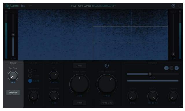
The Repair controls help to remove <u>clicks</u>, <u>crackles</u>, and <u>clipping</u> from your audio.
